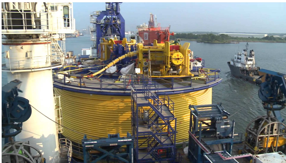
Figure 3-12: Umbilical stored to a reel or carousel
