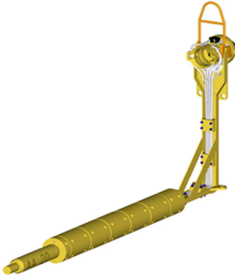
Figure 1-10: Steel Flying Leads [Oilfield]
