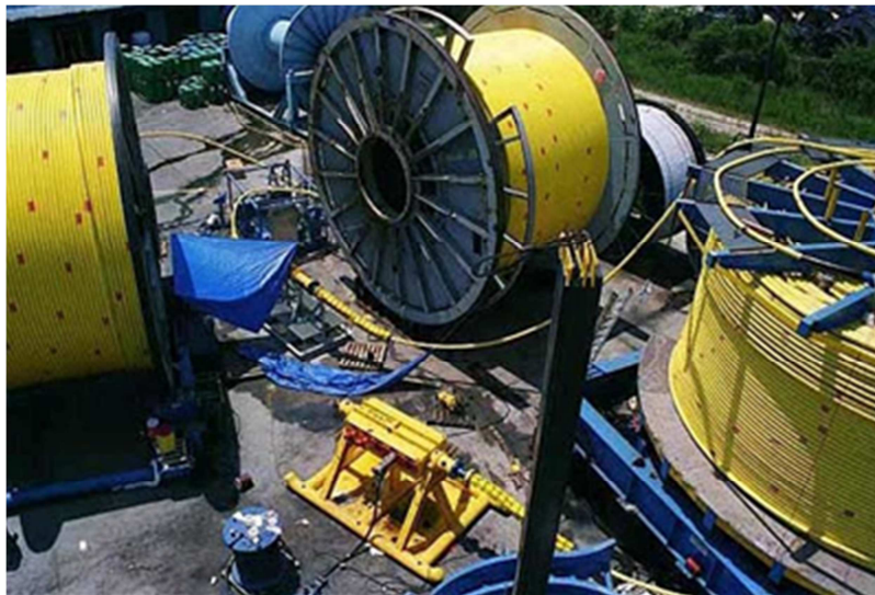
Figure 5-1: System Integration Testing of Control Umbilical
