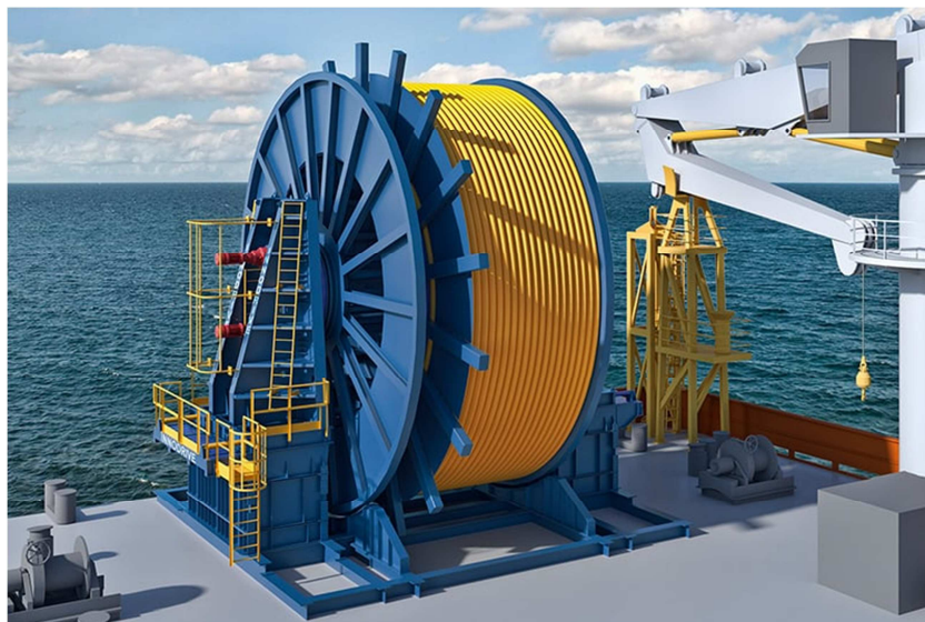
Figure 3-11: Umbilical stored to a reel or carousel
