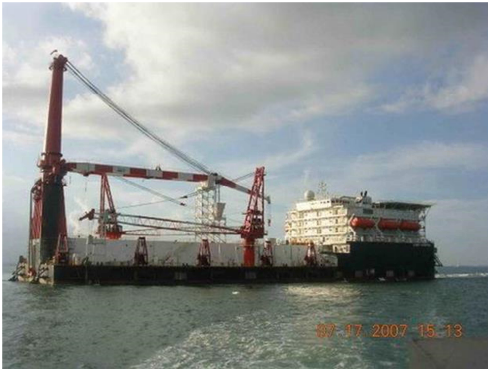
Figure 6.6: Installation barge used for PLEM installation [Zamri]
