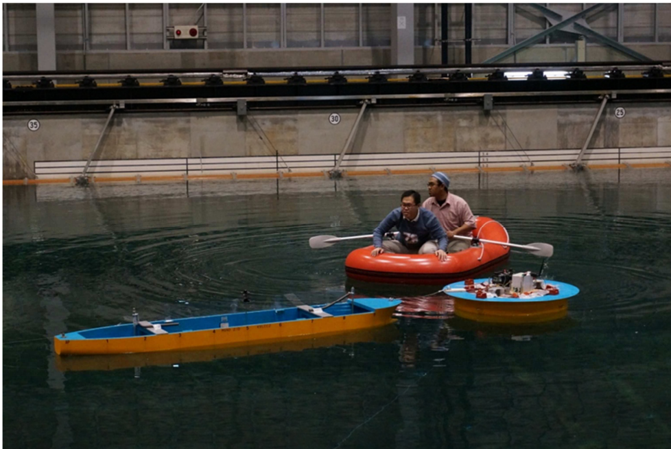
Figure 2.1: Experimental setting up of the tandem arrangement of the rounded-shape FPSO in marine dynamic basin Tank.
