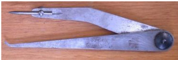
Figure 4.8: Odd leg caliper
