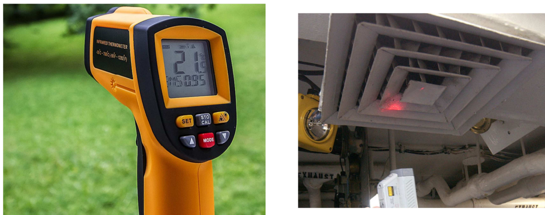
Figure 8.4: An infrared thermometer.
