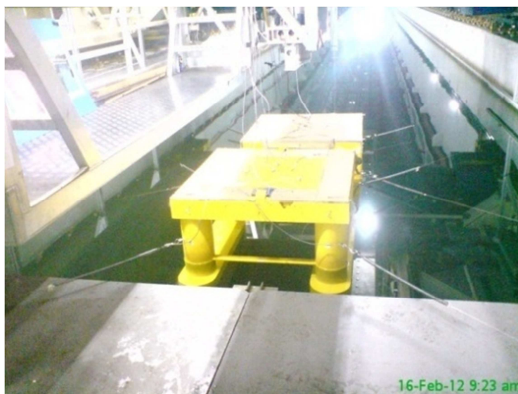
Figure 9.3: TLP and Semi-Submersible set up into towing tank.
