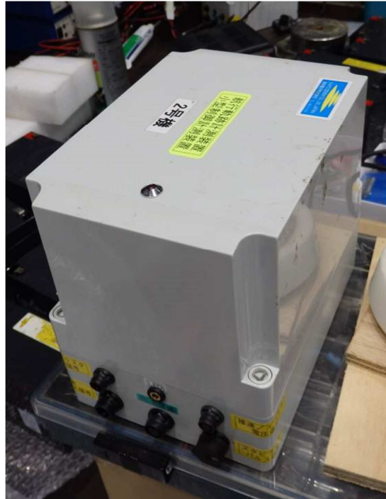
Figure 7.13: Gyroscope to capture model rotational motion of FLNG model
