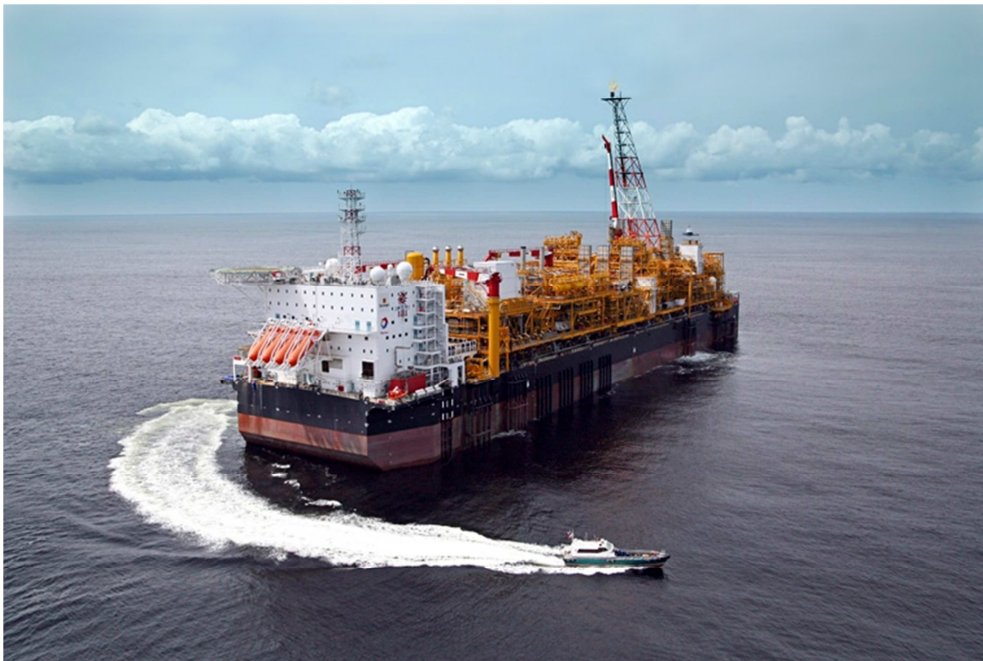
Figure.2.2: Example of Floating Production System [SBS].
