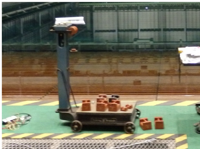
Figure 7.2: Measure the mass of steel blocks before arranged the steel block into round Shape FLNG model
