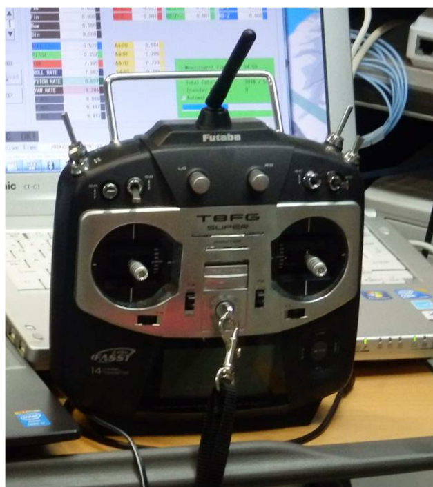
Figure 7.15: Wireless remote controller used to synchronize the start function and stop function of all measurement devices in the experiment
