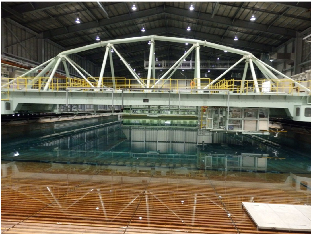
Figure 7.1: The wave dynamic tank used to conduct motion experiment in this research
