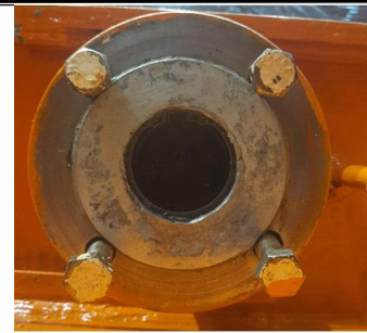
Gambar 7 Oil Vapor Exhaust Pipe
