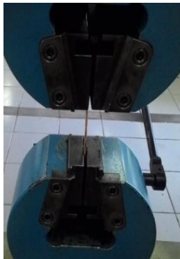
Figure 3 Experimental setup for static tensile test
