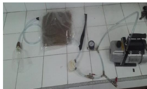
Figure 2 Experimental assembly for manufacturing of composite
