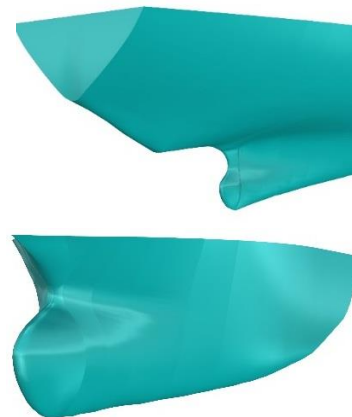
Figure 4 Stern shape and boubous at the stem part after becoming a solid on Rhinoceros and ready to export to Abaqus.
