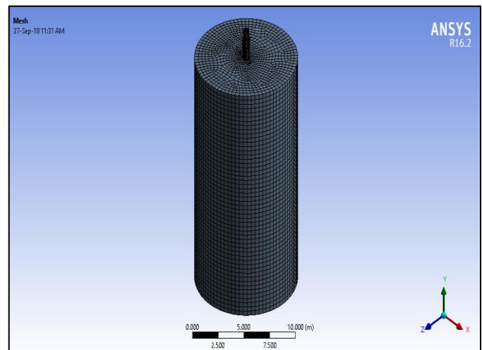
Figure 8: Finite Element Model of the Wellhead-Conductor system with adjoining Soil Domain
