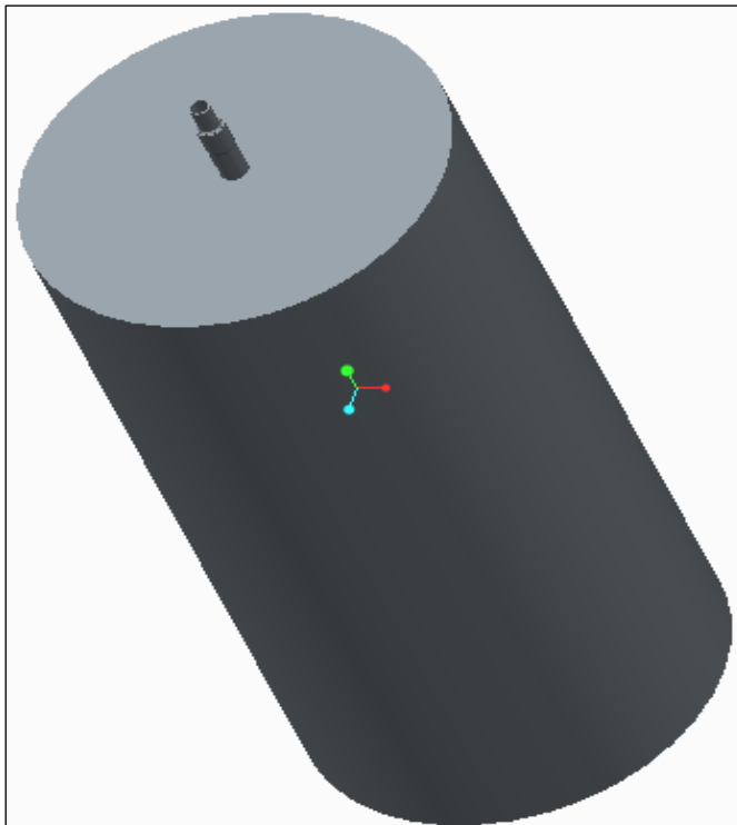
Figure 6: Isometric View of the Global Model of Wellhead-Conductor System with the adjoining Soil Domain
