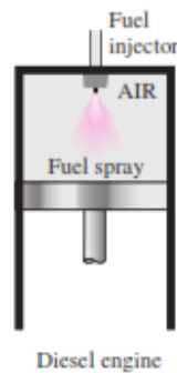
Figure 1. In diesel engines, the spark plug is replaced by a fuel injector, and only air is compressed during the compression process.
