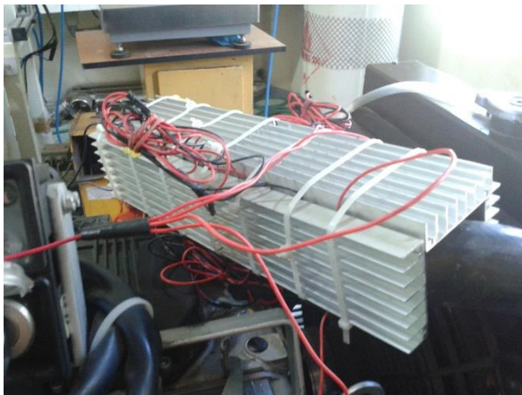
Figure 5 : TEG construction with 20 semiconductors.
