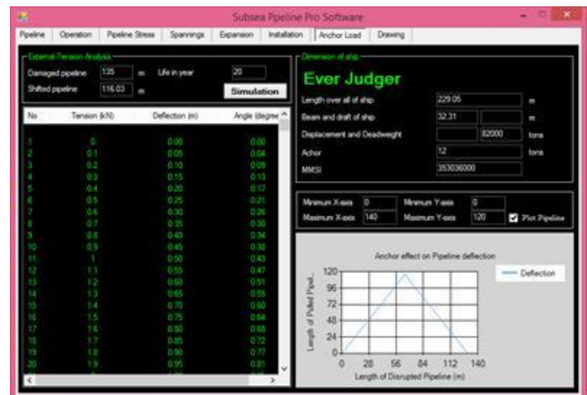
Figure 10: Anchor effect on subsea Pipeline
