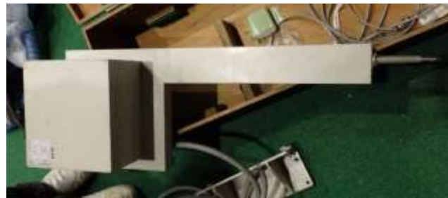
Figure 11: servo-type wave height measurement device (Servo 式波高計) used to measure generated wave height.
