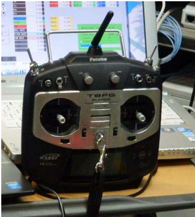
Figure 12: Wireless remote controller used to synchronize the start functioning and stop functioning of all measurement devices in the experiment.
