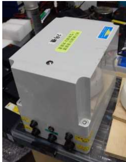
Figure 10: Gyroscope to capture model rotational motion of FPSO model.
