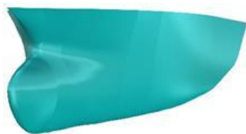
Figure 5: Stern shape and bulbous at the stem part after become a solid on Rhinoceros and ready to export to Abaqus.
