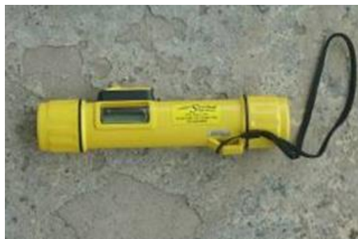
Figure 5: Speedtech SM-5A Depthmate Portable Sounder
