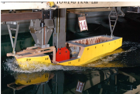
Figure 10: The resistance model testing in TT
