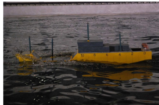
Figure 3: The seakeeping model testing in MOB
