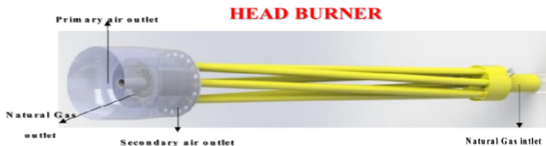
Figure 3: Non-premixed combustion burner head assembly
