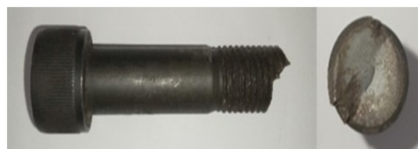
Figure 1: Bolt M20 ×110ISO 4762 as a fastener for the screw conveyor and gearbox that broke in 2024
