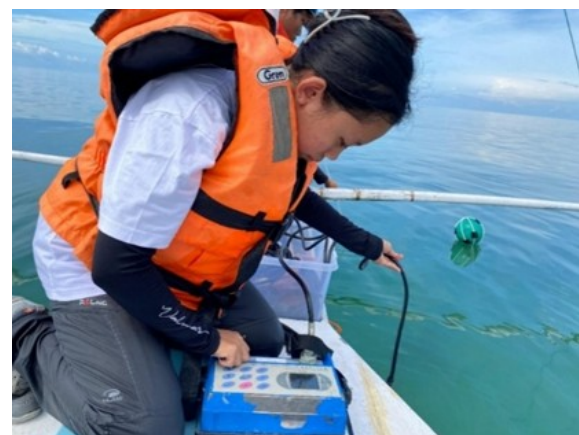
Figure 11: Temperature measurement using a Salinometer
