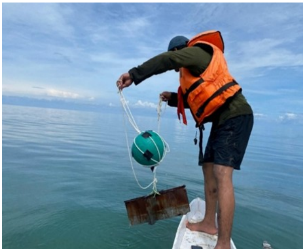
Figure 4: Determination of the current direction using the approximate ball method
