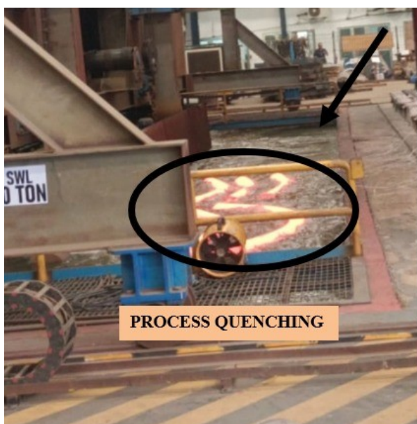
Figure 4: Post bend heat – quenching process
