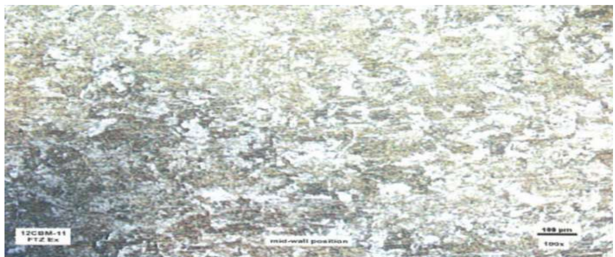
Figure 10: FTZ extrados magnification 100 x
