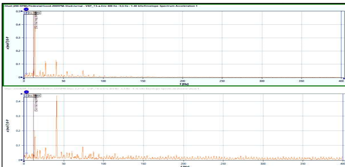
Figure 9: Envelope spectra at 200 RPM with stud mounting: baseline bearing (top) and defected bearing (bottom)
