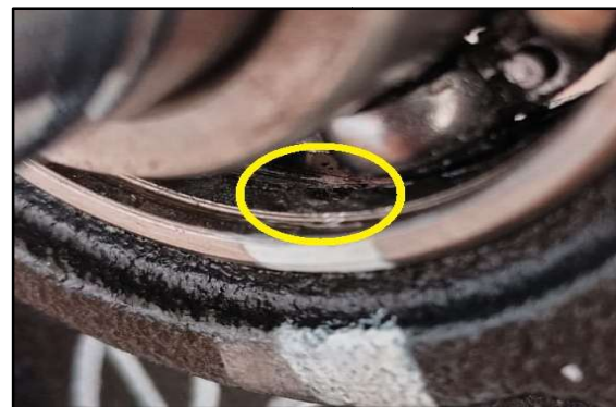
Figure 2: Artificially induced defect on the outer race of UCPH206 bearing
