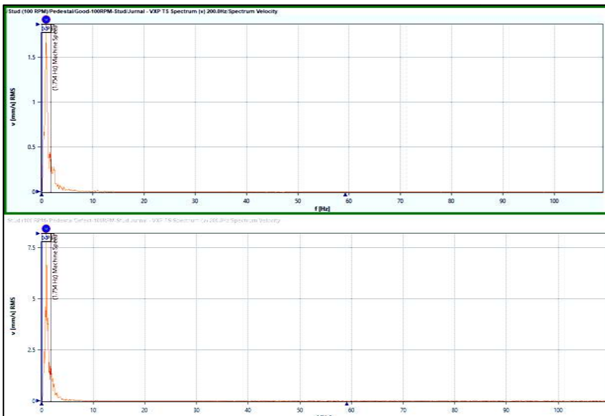
Figure 7: Velocity spectra at 100 RPM with stud mounting: baseline bearing (top) and defected bearing (bottom)
