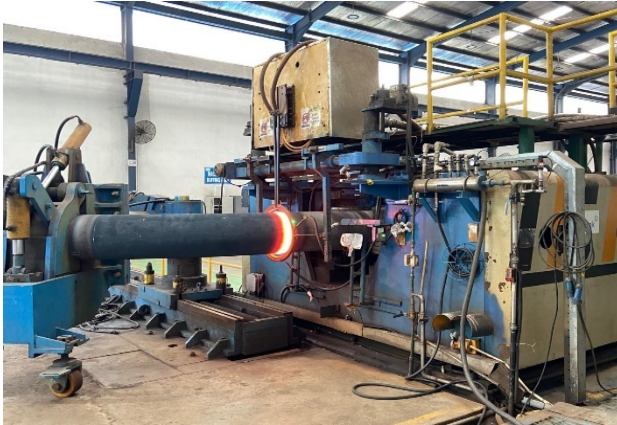
Figure 3: Hot induction bending process
