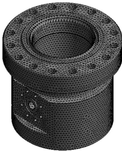
Figure 4: Mesh generates of the casing head
