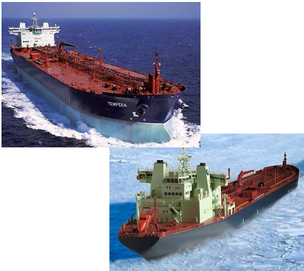
Figure 1: Double acting ship run head in open water and astern in ice condition [marine.com].
