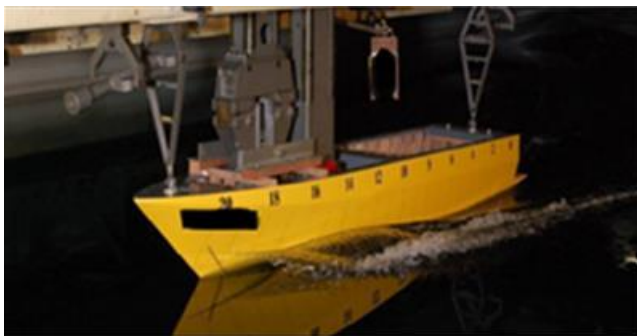
Figure 9: Testing of fast patrol ship resistance model in Towing Tank IHL-BPPT
