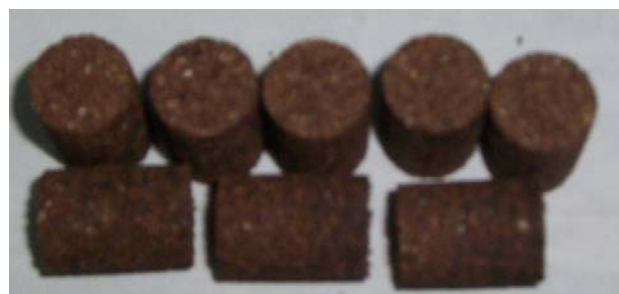
Figure 2: CNS pellets using starch as a binder.
