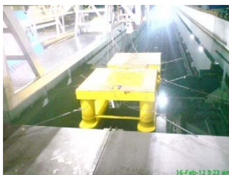
Figure 3: TLP and Semi-Submersible set up into towing tank.
