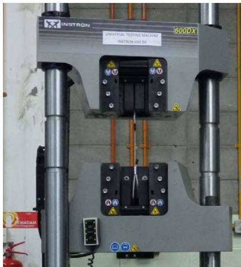
Figure 5: Wire rope tensile experiment setup
