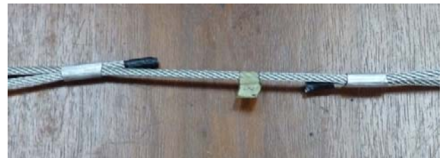
Figure 4: Wire rope with end termination.
