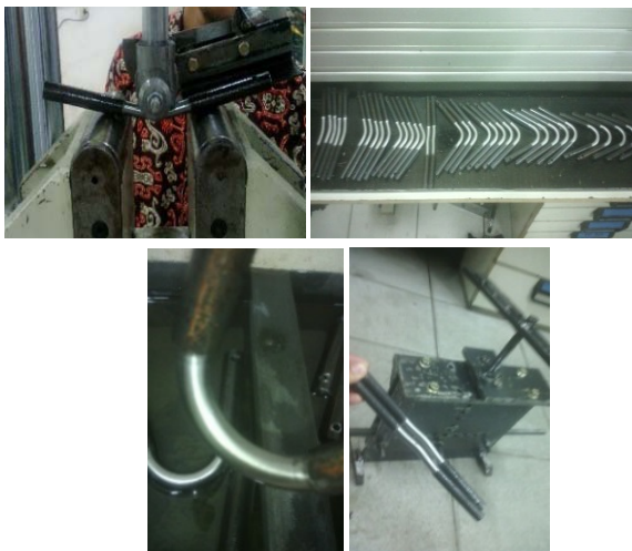
Figure 8: Bending and straightening
