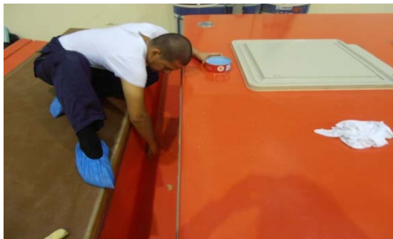
Figure 7: Mould Preparation – Clean and Waxing
