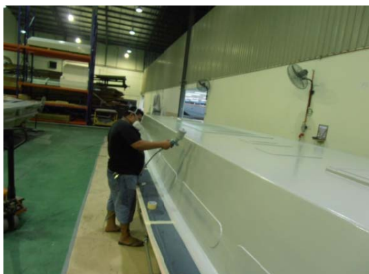
Figure 8: Mould Preparation - Gelcoat Process
