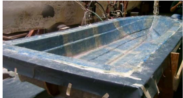
Figure 1: Hand Layup Method
