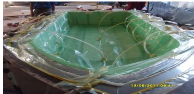
Figure 2: Resin infusion setup
