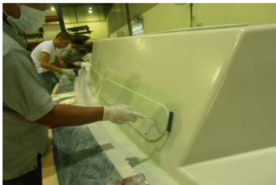
Figure 9: Mould Preparation – Skin Coat Process
