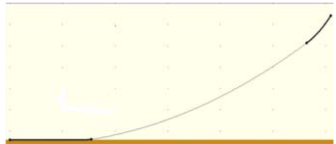
Figure 1: Mooring line profile
