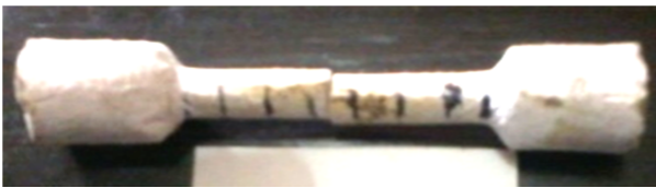
Figure 5: Fractured Tensile Test Specimen of Artificial Bone
