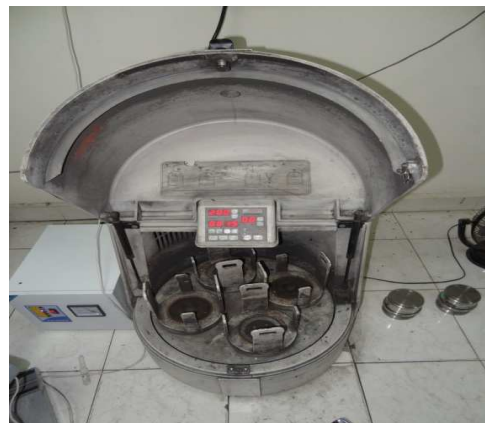
Figure 1. Fritsch Pulverisette(5) – High Energy Ball Mill
