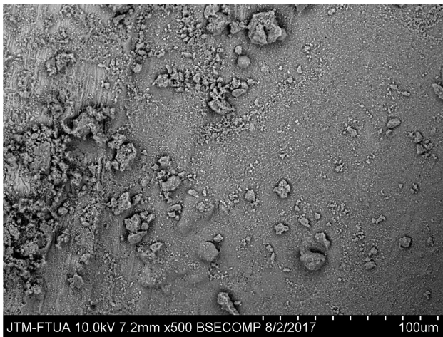
Figure 2: SEM assessment of hydroxyapatite bilayer coating at surface Ti6Al4V ELI screw
