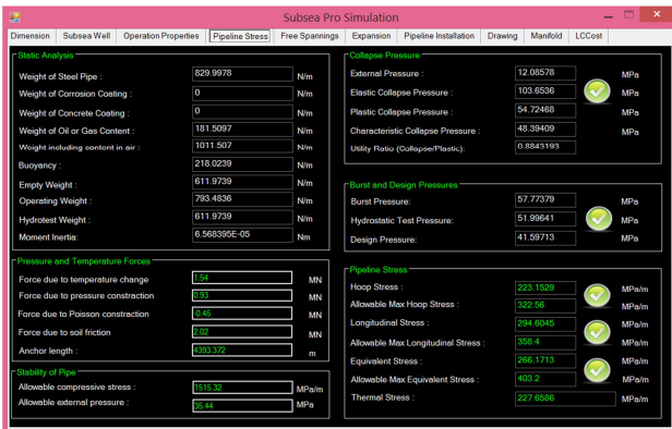
Figure.12: Pressure and Stress of production flowlines.
