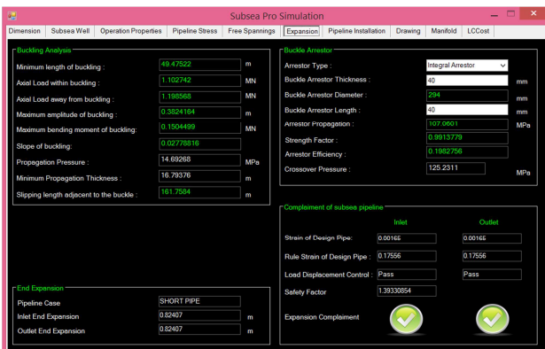
Figure.18: End expansion safety factor of gas injection pipelines.
