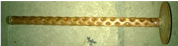
Figure 3: g) Photograph of the tube with staggered dimples
