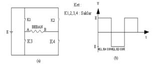
Figure 2: (a) The circuit of full-bridge inverter, (b) Signal wave output [10].
