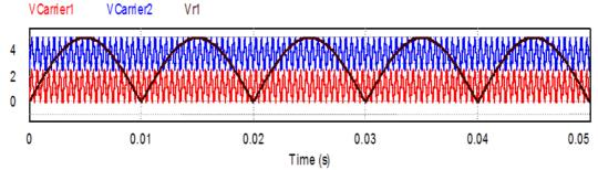
Figure 6: The signal carrier and reference of single-phase five-level inverter.
