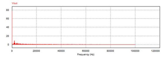
Figure 10: The harmonic spectra of single-phase five-level inverter voltage wave form.
