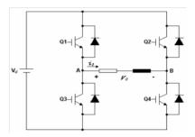
Figure 4: The circuit of conventional rectangular full-bridge inverter [6].
