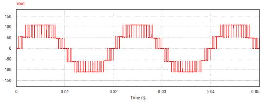
Figure 8: The output voltage of single-phase five-level inverter.
