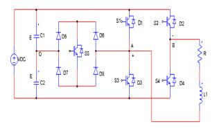
Figure 5: The circuit of single-phase five-level inverter.
