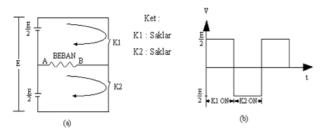
Figure 1: (a) Single-phase half-bridge Inverter, (b) Signal wave output [10].
