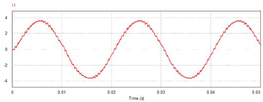
Figure 9: The output current of single-phase five-level inverter.
