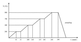
Figure 2: Calcination process step of freshwater snail shell
