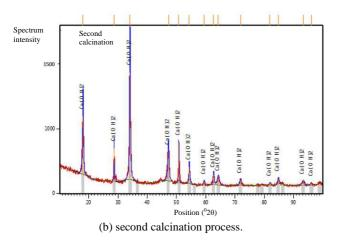
Figure 7. Difractogram of powder of freshwater snail shell.
