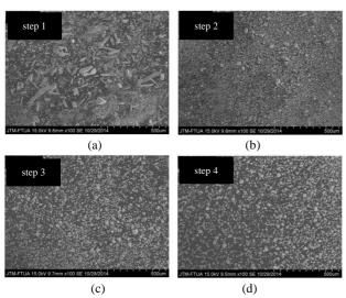
Fig. 3: Size distribution of powder of freshwater snail shell with magnification about 100x; (a) powder of step 1, (b) powder of step 2, (c) powder of step 3, (d) powder of step 4.
