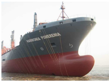
Figure 4: Bulbous bow for common tanker
