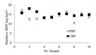
Figure 6: Hardness number of CBP and PBP in wet condition
