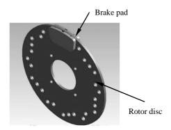
Figure 2: Brake pad and rotor disc
