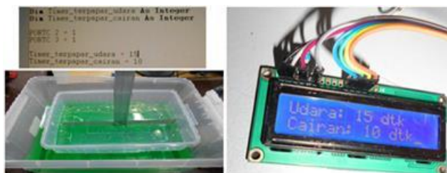
Figure 6: Result of timing exposed to the air 15 second and exposed to the liquid 10 second.
