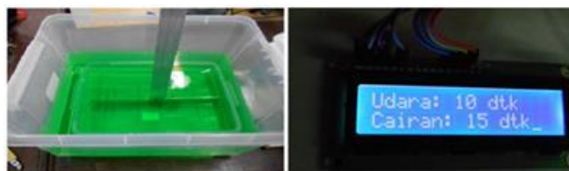
Figure 7: Result of timing exposed to the air 10 second and exposed to the liquid 15 second
