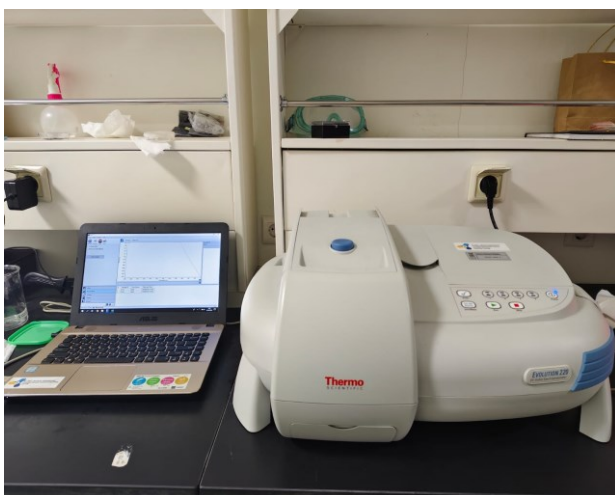
Figure 5: Testing process using UV-Vis Spectrophotometry
