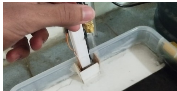
Figure 19: Condition of water pump turning on when temperature is above 34 degrees celsius
