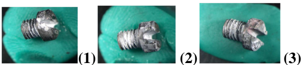
Figure 1: Screws sample of Voltages variation (1). 3V, (2) 5V, (3) 7V
