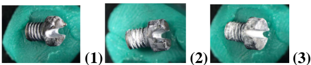
Figure 2: Screws sample of Coating Time variation (1) 3M, (2) 5M, (3). 7 M
