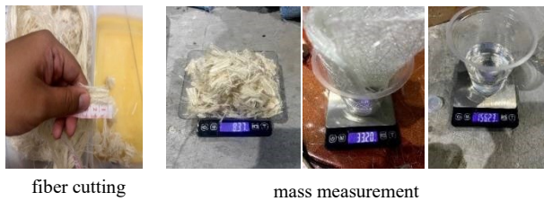
Figure 4: Mass measurement of fiber and matrix
