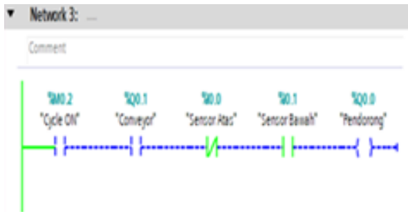
Figure 38: Control program 2: Moving the cylinder
