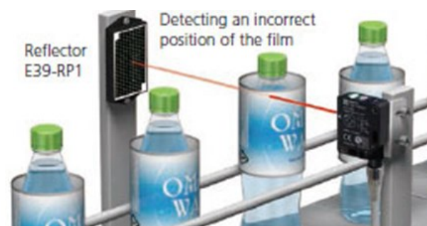
Figure 11: Position of E3S-DB sensor and E39-RP1 reflector for bottle detection.
