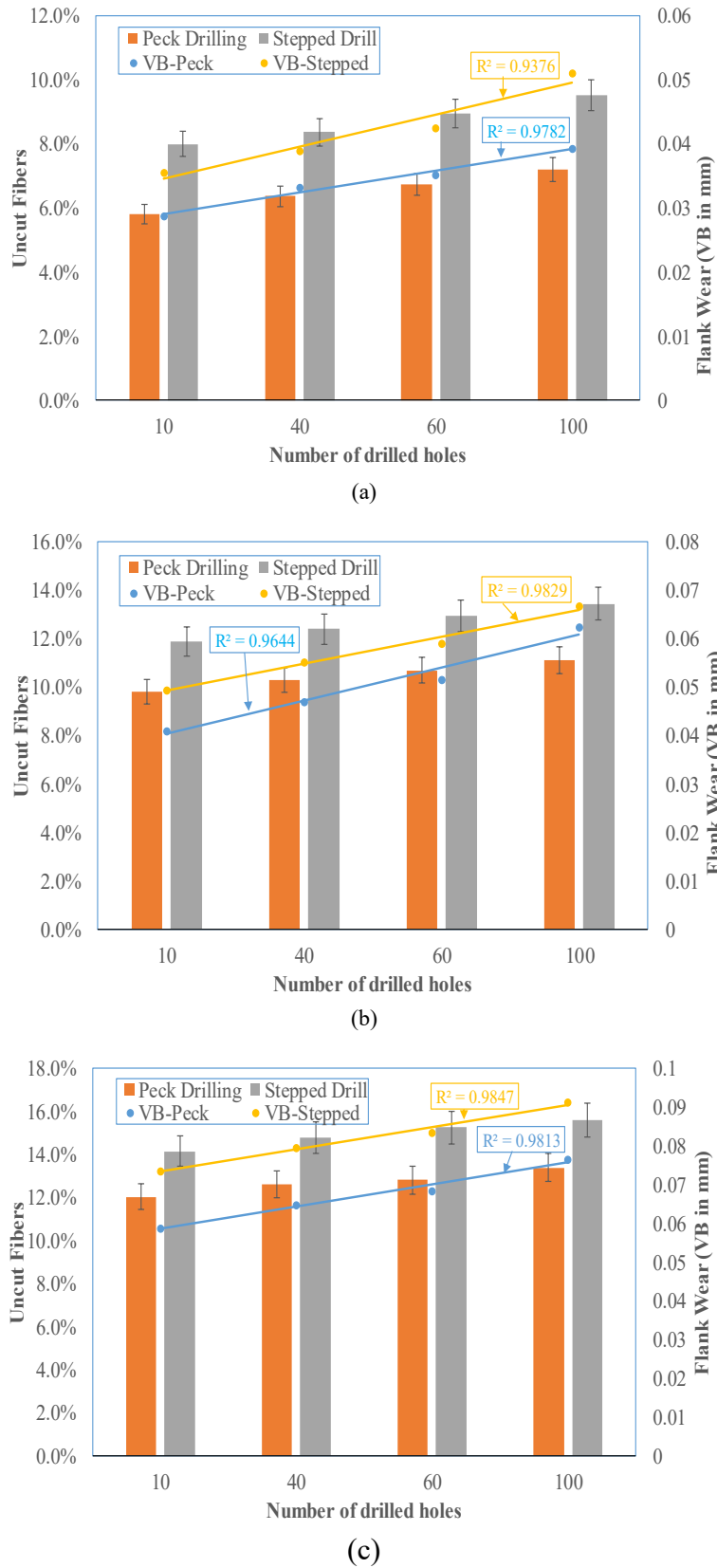
Figure 6: Progression of percentage area of uncut fibres as consequences of tool wear progression
