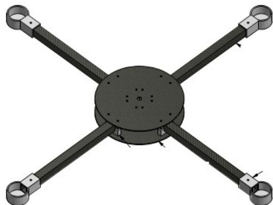
Figure 10: Design result of quadcopter frame
