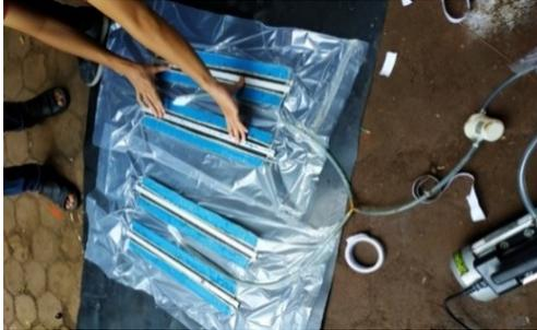
Figure 6: The manufacturing process of the quadcopter arms
