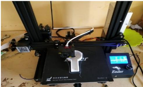
Figure 8: The 3d printing process of motor mounting
