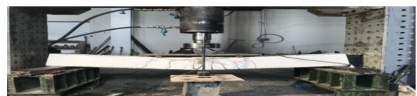
Figure 6: Beam B 0 after loading operations
