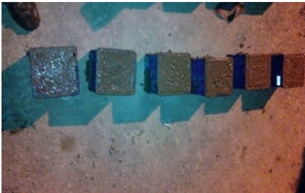
Figure 4: The cubic samples for determining concrete compressive strength
