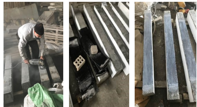
Figure 5: Performing preparation operations and adhering FRP sheets to the samples
