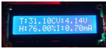
Figure 7: Data display on 16*2 LCD
